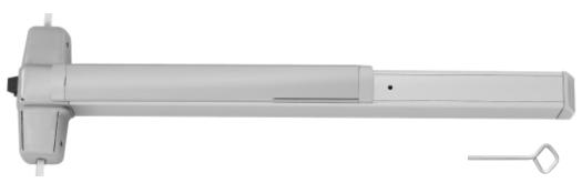
**9857/9957 three-point latching device** for all types of single or double doors, UL listed for Panic Exit Hardware. Devices are ANSI A156.3 – 2001 Grade 1. Covers stock hollow metal doors with 86 or 161 cutouts. The 9857 device has a smooth mechanism case and the 9957 device has a grooved case. The three-point latching device is non-handed except when the following device options are used: SD (Special Dogging), or SS (Signal Switch). See Opposite page for available outside trim and functions.
